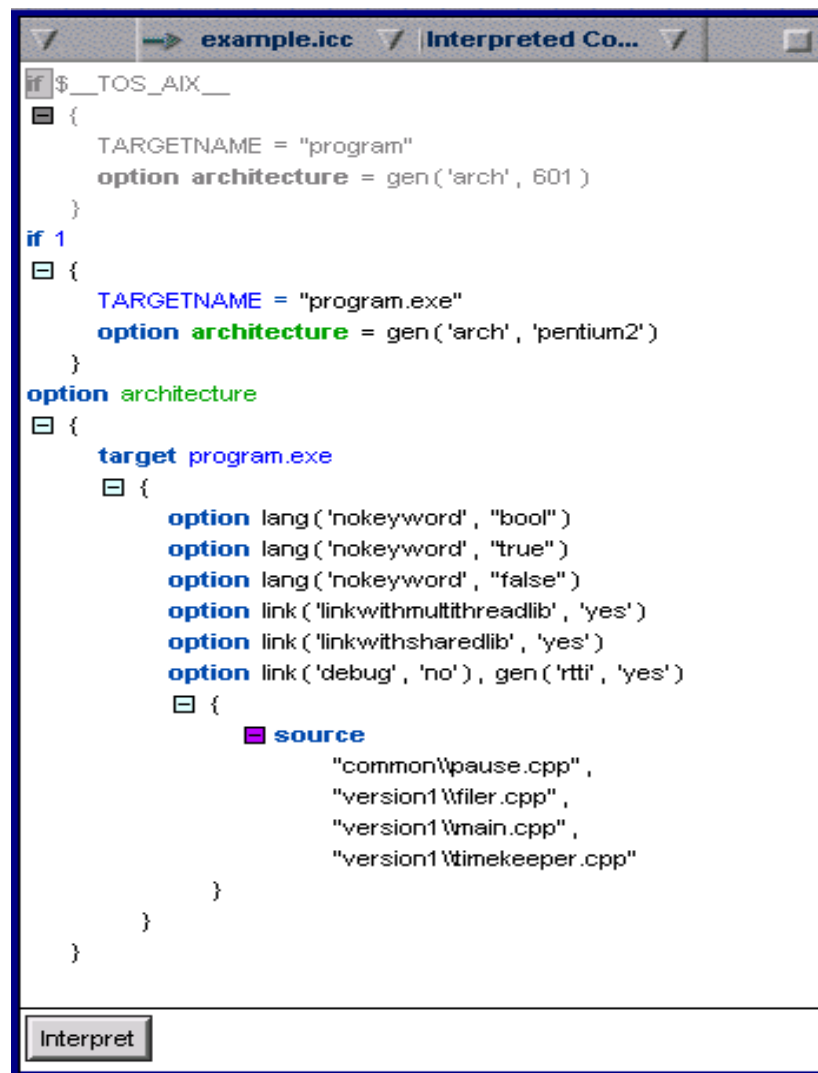
Figure 20. Interpreted ("preprocessed") configuration file
